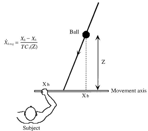
**Fig. 1** Diagram representing the current lateral distance. In Peper et al.’s (1994) strategy, the *subject* must cover the current lateral distance  $X_h - X_b$  within the (first-order) time remaining until the *ball* reaches the interception point  $TC_1(Z)$
