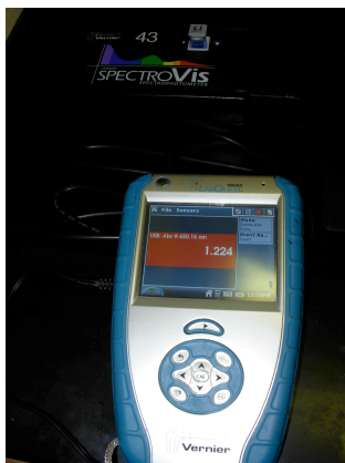
Figure 5: LabQuest, SpectroVis Spectrophotometer, and 3 mL cuvette
